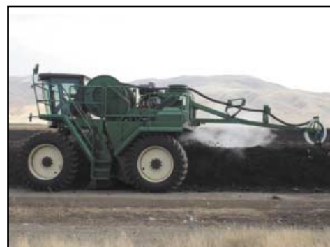
SP-170 equipped with the hose reel system
