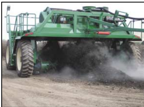
The SP-170 Aeromaster Drum is especially designed to turn outside in and inside out, treating every particle in the windrow.
