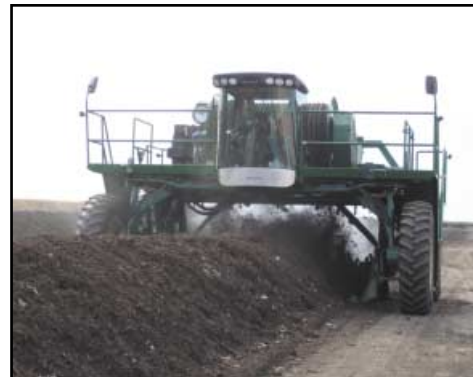
The unique water and inoculation system assures even moisture to every particle as the turner moves through the windrow.
